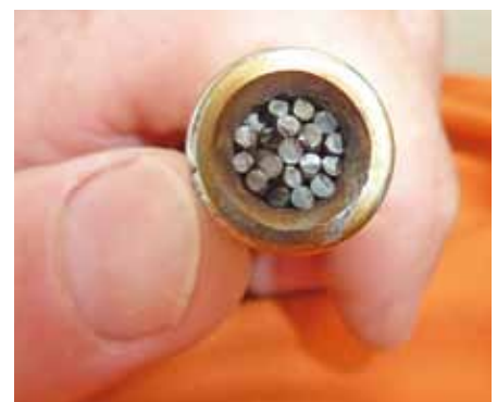
The break was clean and corrosion-free
