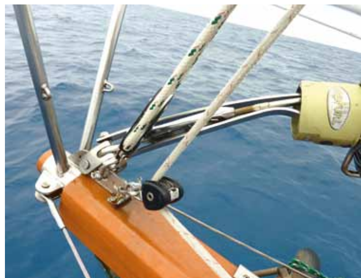
Two halyards led from the masthead to the bowsprit, through blocks and then aft, secured the mast after our forestay snapped
